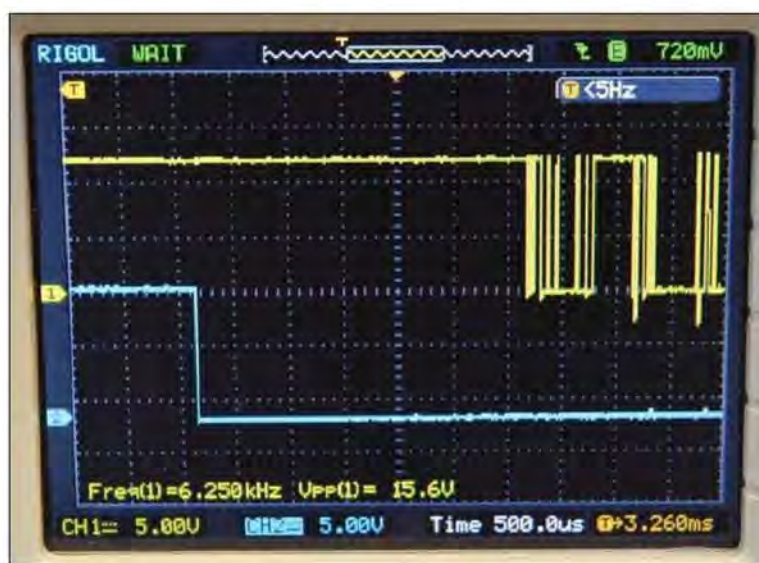
Figure 1 — Timing comparison (0.5 ms per division horizontally) of a Jennings RJ1a (bottom curve) and a Gigavac G41c (top curve) vacuum relay. The RJ1a contact closes in 1.2 ms and shows no contact bounce. In contrast, the G41c contact closes in about 5.9 ms after appreciable contact bounce.
